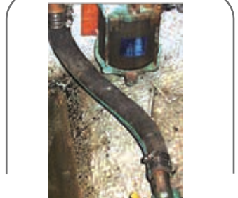
Clamps installed with screw tightening heads in line. It is recommended to offset as see below.
