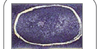
Hose with cover charred area from high heat or extreme aging due to heat or ozone
