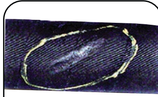
Hose cover melted due to contact with high heat of hot engine parts
